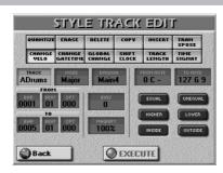
The CHANGE VELO function allows you to modify the dynamics (called "velocity") of a track or excerpt. See p. 185 for details. Only note events can be changed.
